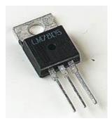
Many of the fixed voltage regulators have 3 leads and look like power transistors, such as the 7805 (+5V 1A) regulator shown on the above. If adequate heat sinking is provided then it can deliver up to maximum 1A current. For an output voltage of 5v-18v the maximum input voltage is 35v and for an output voltage of 24V the maximum input voltage is 40V.For 7805 IC, for an input of 10v the minimum output voltage is 4.8V and the maximum output voltage is 5.2V. The typical dropout voltage is 2V.
