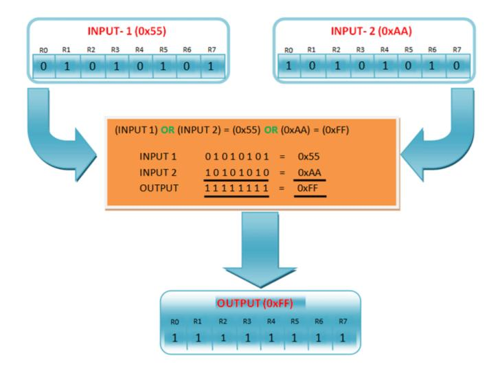
The CPU takes values from two input registers INPUT-1 and INPUT-2, performs the logical operation and stores the value into the OUTPUT register. All this happens in 1 execution cycle.
